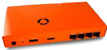
Exostiv Labs designs innovative solutions for FPGA debugging. EXOSTIV IP uses the MGTs (Multi-Gigabit Transceivers) to flow captured data out of the FPGA to an external memory. EXOSTIV IP supports repeating captures of up to 32,768 internal nodes simultaneously at the FPGA's speed of operation (16 data sets x 2,048 bits\*).
